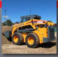
**EXTRA LONG WHEELBASE** • enhances machine stability when lifting and loading providing a smoother ride over rough terrain.
