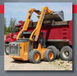
VERTICAL BOOM DESIGN A delivers extended reach and high lift heights for easy truck loading and material handling in a vertical path. (near vertical path on 2700V NXT2 and 3300V NXT2)
