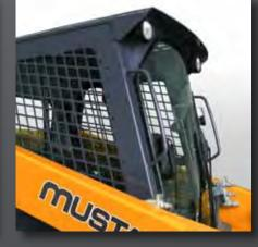
**EXCELLENT VISIBILITY** A to the sides, rear and front is achieved with a unique, low-profile boom design. A roof window allows the operator to view the quick-attach when the lift arm is fully raised.
