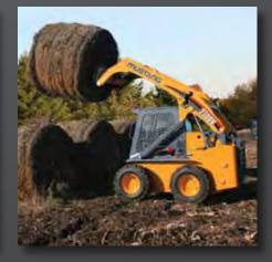
HEAVY-DUTY CHASSIS A provides excellent weight distribution, enhancing machine stability. A rear bumper and counterweight on the model 3300V NXT2 adds protection and towing capability.
